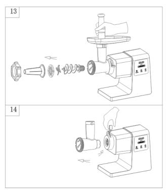
1. Before you clean the appliance, switch the appliance off and remove the plug from the socket.Remove the pusher and the
